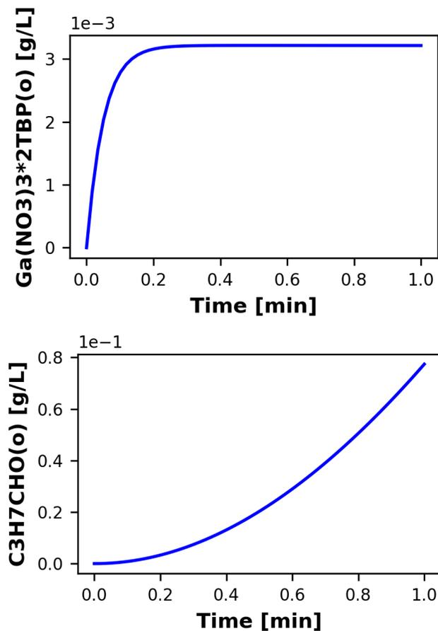
Fig. 2. Examples of simulated species concentration in the organic phase; bottom plot shows butanal as a degradation product of TPB.
