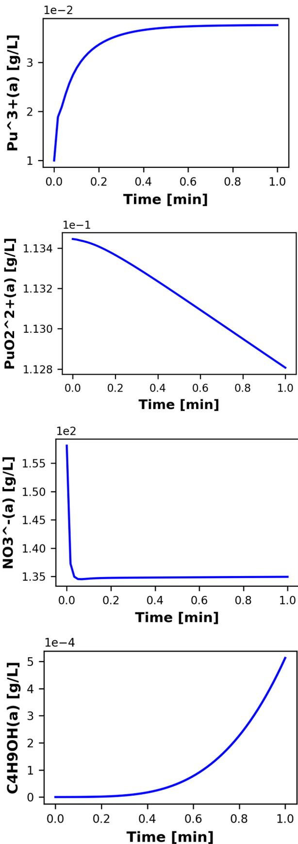
Fig. 1. Examples of simulated species concentration in the aqueous phase; bottom plot shows butanol as a degradation product of TPB.
