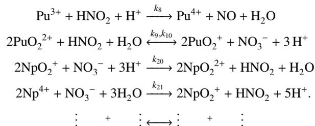
The complete set of actinide redox reactions add 29 reactions and 19 species to the overall reaction mechanism.
